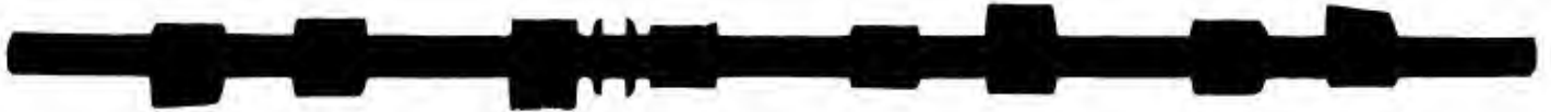
LOCOMOBILE CAMSHAFT WITH INTEGRAL CAMS, FORGED IN ONE PIECE, HARDENED AND GROUND.
